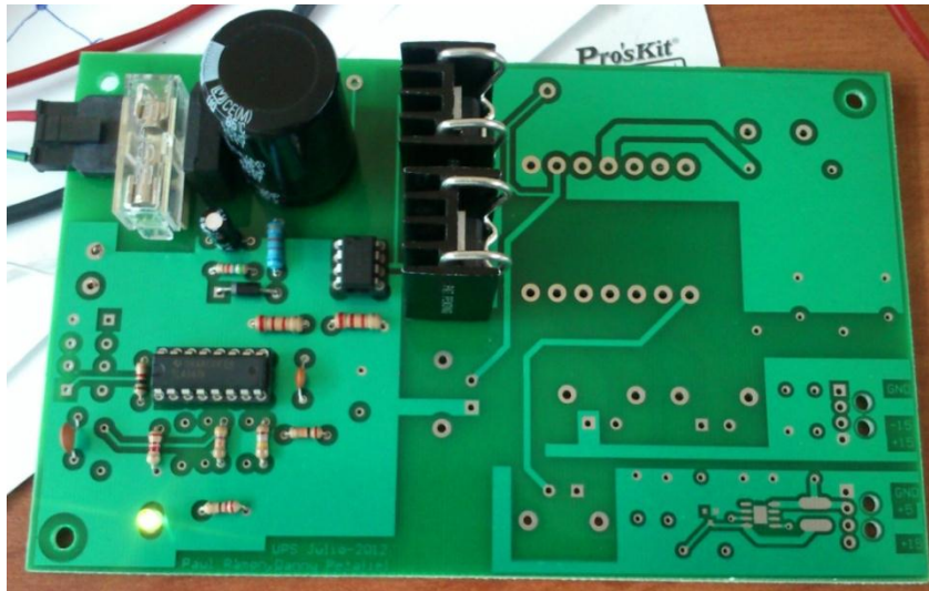
Figura 3.10: Montaje de driver e IGBT's
