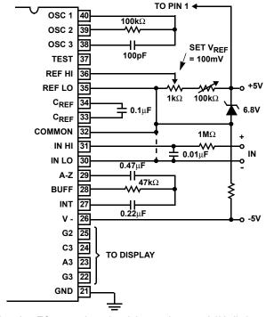
Since low TC zeners have breakdown voltages  $\sim$  6.8V, diode must be placed across the total supply (10V). As in the case of Figure 12, IN LO may be tied to either COMMON or GND.
