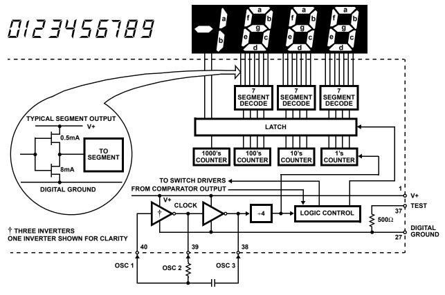
FIGURE 8. ICL7107 DIGITAL SECTION
