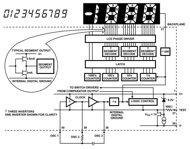
FIGURE 7. ICL7106 DIGITAL SECTION
