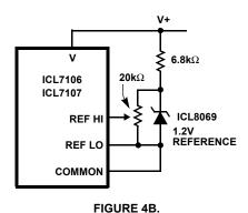
FIGURE 4. USING AN EXTERNAL REFERENCE
