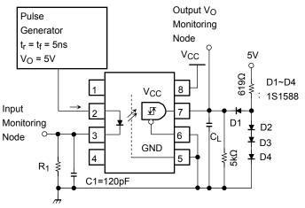
${\sf C}_1$  is peaking capacitor. The probe and jig capacitances are include in  ${\sf C}_1$ .  ${\sf C}_L$  is approximately 15pF which includes probe and stray wiring capacitance.
