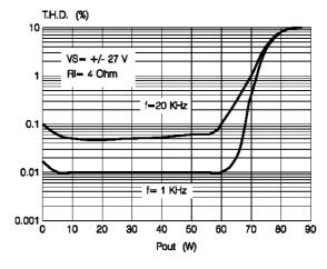
Figure 8: Distortion vs. Frequency
