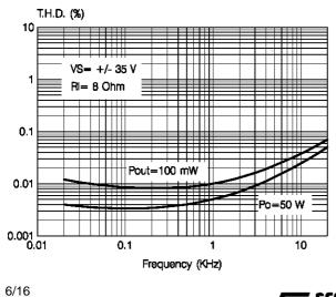
Figure 4: Distortion vs. Output Power
