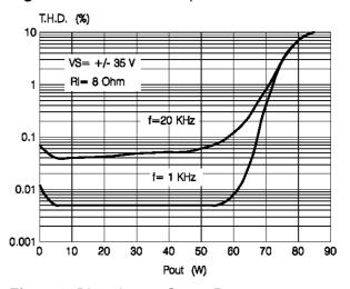
Figure 6: Distortion vs. Output Power
