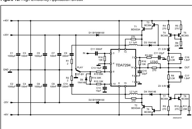
Figure 18: High Efficiency Application Circuit
