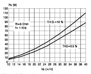
Figure 5: Output Power vs. Supply Voltage
