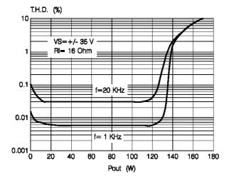
Figure 27: Distortion vs. Output Power
